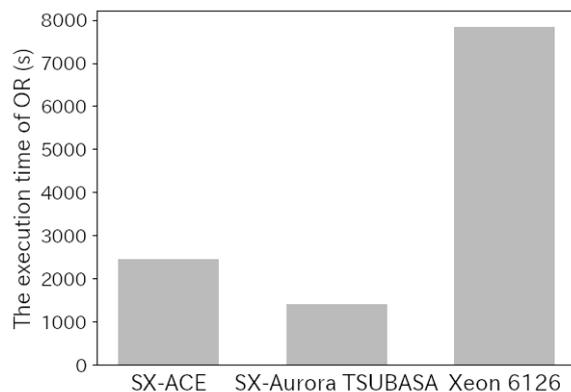
**Figure 15.** The execution time of OR on the SX-ACE system, the SX-Aurora TSUBASA system and the Xeon 6126 system
