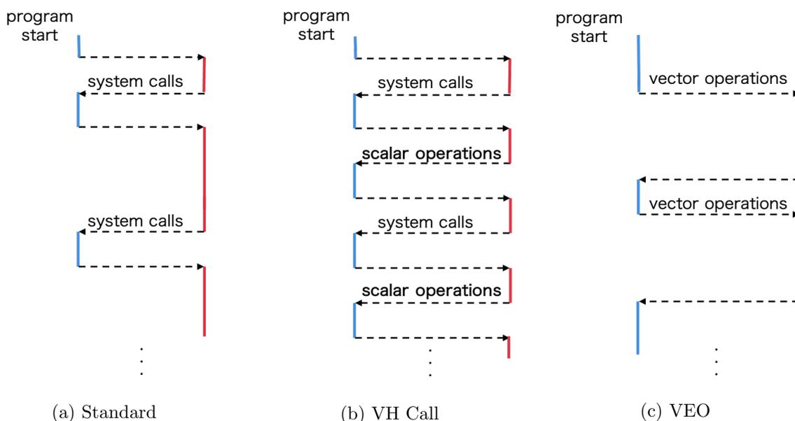
Figure 3. Three execution models of the SX-Aurora TSUBASA
