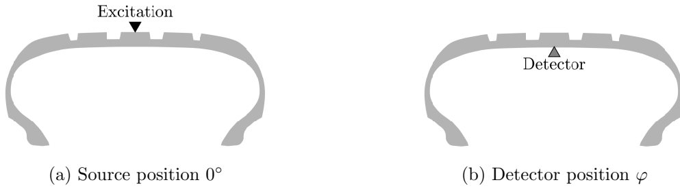
Figure 2. Tire profiles at the source and the detector azimuth positions
