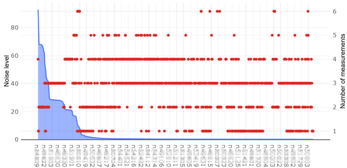
Figure 2. Average noise level at different nodes of a supercomputer. Blue area shows the average noise value for nodes, red dots show the number of noise level measurements on the basis of which the average was calculated
