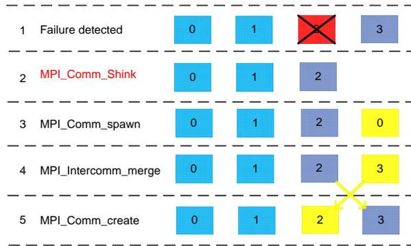
Figure 2. Recovery process of a communicator
