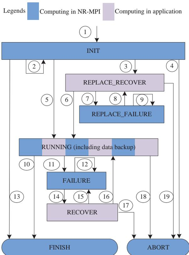
Figure 3. State transition diagram of a NR-MPI process
