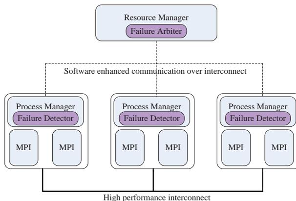
**Figure 1.** Structure of the resource management system of NR-MPI
