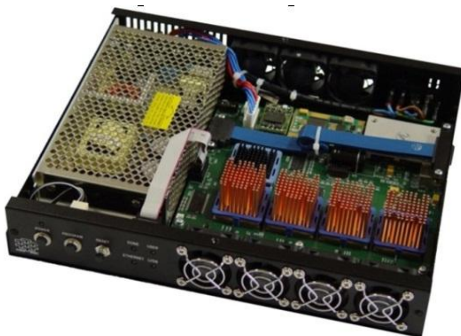
Figure 3. The small-size reconfigurable accelerator of the personal computer
