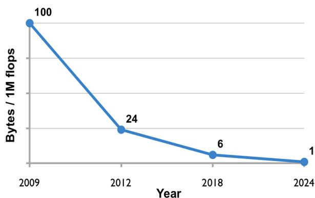
**Figure 8.** Current and expected I/O in bytes per 1 Million FLOPS. Data derived from forecasts on past, current and future HPC systems [12, 25, 31]
