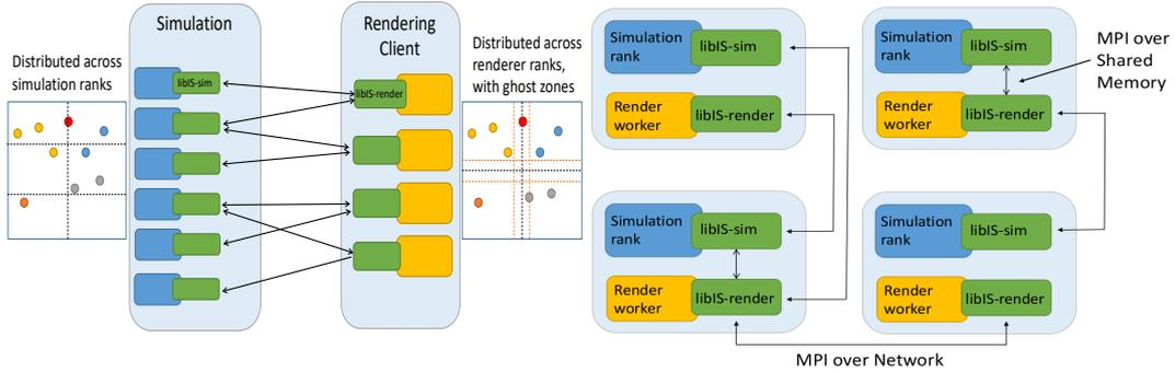
**Figure 2.** Overview of the in situ library, libIS. In our system, data are forwarded via MPI from the simulation to a distributed renderer. When the simulation and visualization are run on different resources (left) all data queries go over the network. When running on the same resource (right), data can be forwarded locally from one process to another on the same physical machine via shared memory or transferred across the network
