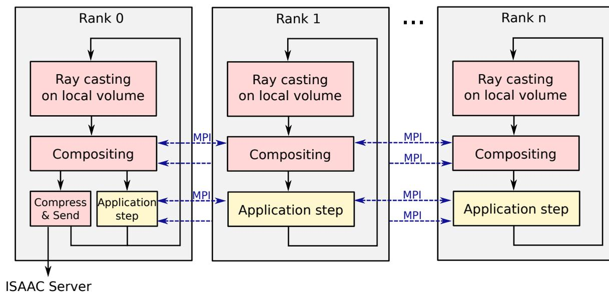
**Figure 1.** The full ISAAC concept. First a local ray casting is done. The resulting images are composited using the interconnect. The whole image is only on the first node in the end. Afterwards the application gets back the focus on every node, but on the first node the image is also compressed and sent to the ISAAC server in parallel
