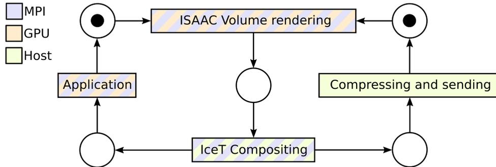
**Figure 5.** As ISAAC and the HPC application work on the same hardware accelerator and both use MPI, they cannot be executed in parallel. Only compressing and sending the final image is invariant of the application and MPI and can run in background while the application continues. Only if both concurrent tasks finish, the next frame can be rendered
