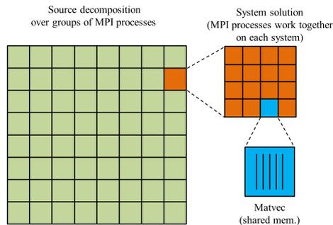
**Figure 1.** Layers of parallelism on a hybrid cluster
