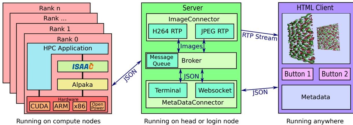
**Figure 4.** ISAAC consists of a library running integrated with the application on the compute nodes, a server running on one the head or login nodes, and an arbitrary amount of clients running anywhere. With this a connection between the compute nodes and the outside of the cluster can be established. Furthermore, the server can compress the data for slower networks
