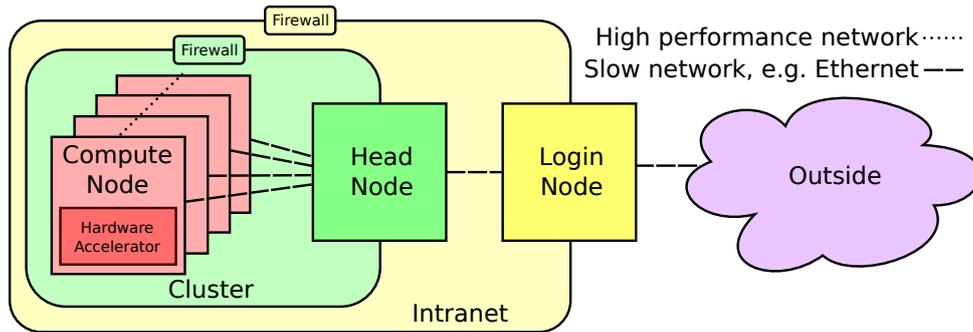
**Figure 3.** Simplified design of a typical cluster with multiple firewalls. The only connection between the compute nodes and the outside (e.g. the Internet) is over the cluster’s head and login nodes. A high performance network can only be assumed between computation nodes. Green shows the cluster, yellow the intranet of the site, and purple the outside
