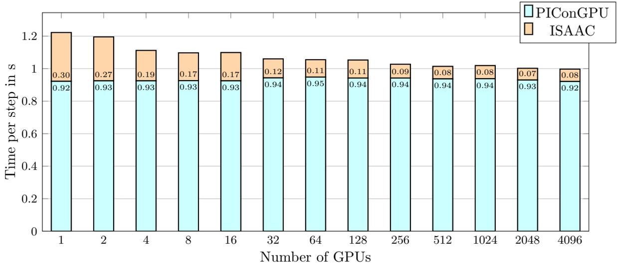
**Figure 6.** PIConGPU with ISAAC running on up to 4096 Nvidia Tesla K20X GPUs ( $\sim 16.2$  PFLOPS/s theoretical peak performance, single precision) on Piz Daint simulating a Kelvin-Helmholtz instability. Every GPU node simulates a volume of  $128^3$ . Adding more GPUs increases the global, simulated volume. PIConGPU shows perfect weak scaling [6], while ISAAC gets faster as the resolution of the image per GPU shrinks and thus the number of needed ray casting rays
