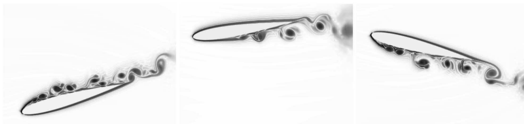
Figure 1. Instantaneous vorticity magnitude for different phase angles of the flapping foil
