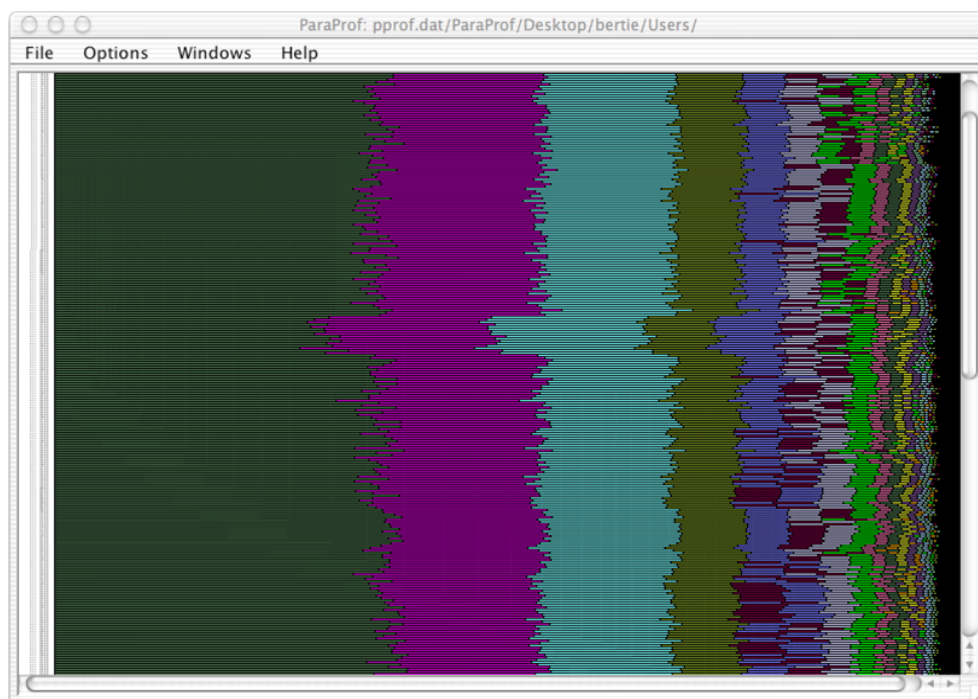
Figure 1. TAU main profile window. Each line shows a flattened histogram of a selected performance metric for a specific thread or task. The different colors represent the different program regions (e.g., functions, loops, parallel sections, etc.). The display allows to get a quick overview via comparing the differences/commonalities of the different threads/tasks. Clicking on a line label brings up more detailed information about the selected thread or task. Clicking on a colored region brings up more detailed information about the selected program region. The menu bar allows to choose the performance metric shown or to launch further, more detailed displays like a call-graph or communication matrix display. Results from larger performance experiments can be more easily analyzed with the 3D displays of TAU, see fig. 2.
