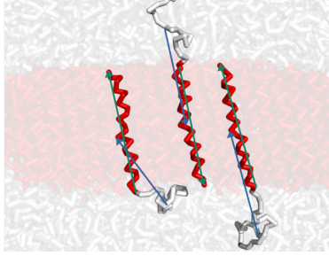
(a) Schematic representation of several molecules of the helix-coil diblock copolymer within the lamella, obtained in [19]
